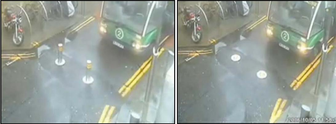
**Example of an Automated Bollard System for Special Vehicle Access**
